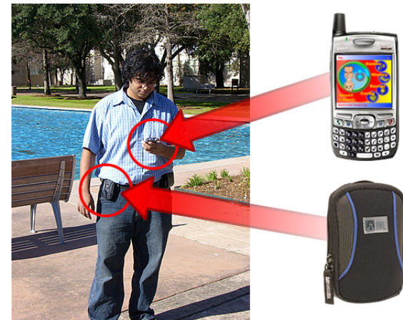
figure 1. User wears activity sensor at his waist and holds a Palm Treo PDA at his palm. The devices are indexed in the right panel, where the form factors are evident.
